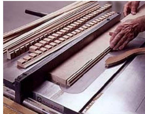
9--Cut the ogee moldings on the edge of a wide board, then rip the molding off the board on the table saw.
