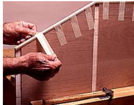
4--The edge banding is glued, and held in place using masking tape. A pair of brads in each band keeps it from slipping.
