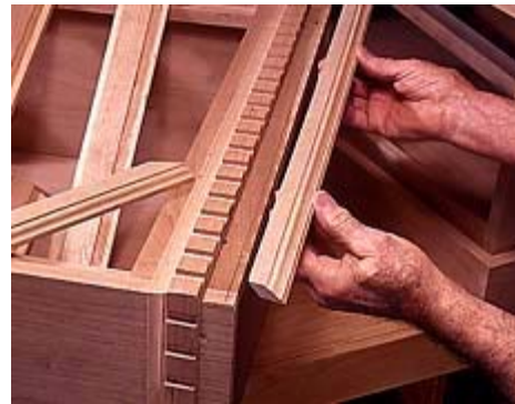
10--The ogee molding above the dentil is held in place with glue, and nails driven into the molding below.
