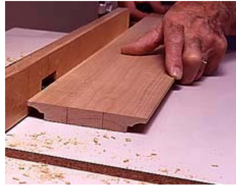
8--Cut the molding on the lower edge of the dentil molding using a router table and a cove raised-panel bit.
