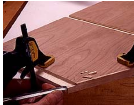
5--The edge banding blocks the rabbet at the top of the lower case. Use a chisel to pare away the edge band at this point.
