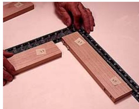
12--With dowel centers inserted, press the door parts together while aligning them with a framing square.
