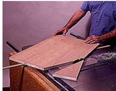
2--To cut the angle on each side panel, slide the guide strip in the miter gauge groove and push the panel through the blade.
