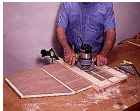
3--Use a router with a straight bit and a parallel fence jig to cut the rabbets and dadoes in the case sides.
