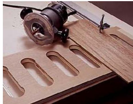
11--Smooth the slots in the butt rest using a flush-trimming bit and a router. Run the router along a fence clamped in place.
