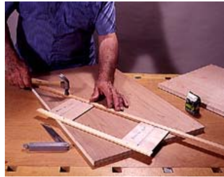
1--Use a strip of wood and a pair of blocks to position the guide strip on the case side. Nail the strip to the panel.
