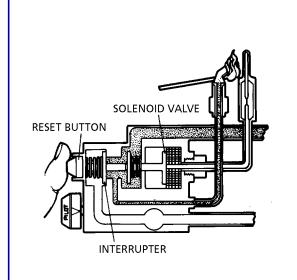
**Thermocouple** usually is in this configuration. Line or tube runs from coupling at control to bracket at thermocouple. Be sure to press reset when re-lighting pilot; drawing shows how solenoid valve works in controls.
