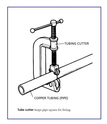
Copper pipe is always 1/8-inch larger than the nominal size. Example: 1/2-inch pipe measures 5/8-inch. outside diameter. The actual inside diameter varies with the thickness of the pipe wall. The thicker the wall, the smaller the inside diameter of the pipe.
