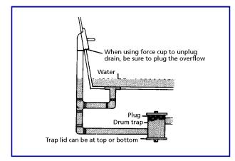
Drum traps are not too common in modern plumbing systems, but your home, especially if it is an older one, may be equipped with them. Look on the bathroom floor under a tile, perhaps. Or the trap may be in the floor in the basement or crawl space. Clean this trap by removing the lid—similar to a clean-out plug or trap as detailed.
