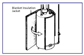
all sizes and are easy to install. In some cases, it is possible to save 10% to 15% of the water-heating energy by adding proper insulation. But when installing the insulation, be sure not to block off needed air vents. That would create a safety hazard. Insulation kits are available.
