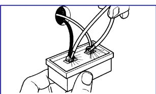
To test a transformer, use a voltage meter, or make a jump wire from 14 or 16 gauge wire as detailed in the text. If you see faint sparks from terminals, the transformer is in working order.
