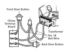
**Sounding device terminals** are marked for proper hookup. Bell wire is not "coded" as such, but you can buy it with different colored insulation which might make terminal hookups easier.
