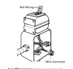
**Turn off housepower** before you connect it to the transformer which is prewired to accept it. Use wire connectors and tape the nuts.
