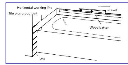
Battens, if needed, above the tub (set at a height of one tile plus grout lines) are left until the adhesive has set. Then remove the battens and fill in the row of tile, cutting the tile if needed. The battens are set to correspond with the tub level, when working from the low end toward the bathtub drain opening.
