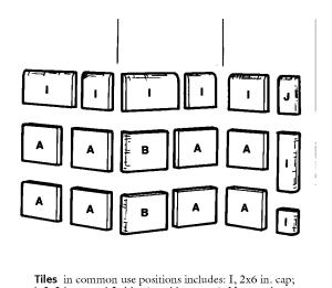
**Tiles** in common use positions includes: 1, 2x6 in. cap; 1, 2x2 in. round 2 sides (outside corner); Note perimeter capping utilizing 2x6 in. caps, cut pieces of 2x6 in. caps, and 2x2 in. round (2 sides) at outside corners.
