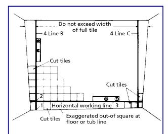
**Before setting tile**, square off the wall using a level and carpenter's square. Then work out the numbers and locations of the tiles that need to be cut to fill out-of-square edges. Almost all wall situations will follow this layout plan. If fixtures will be added, such as soap dishes, towel bars, etc., locate these items at the time of layout.
