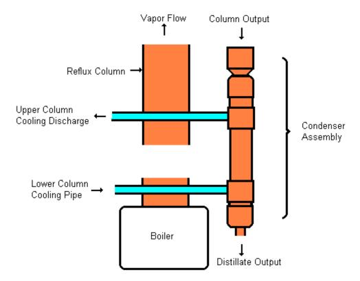
Those are the reasons why the big, jacketed condenser we are going to build for this job is better. Its also happens to be easier to fabricate and more efficient than those condensers which use a coiled tube contained within the distillate output pipe.
