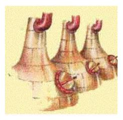
The copper pot stills like the ones shown are reputed to have been in use for over 500 years to make some of the finest Irish Whiskey in the world While the pot still is enormously inefficient, it is uniquely simple and easily adapted for home distillation of everything from essences to whiskey and moonshine.
