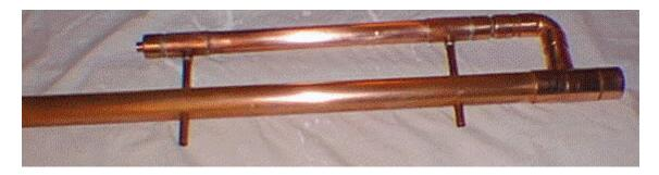
Make sure everything fits OK and aligns well. When you're satisfied, remove the cooling tubes and condenser. Clean up and solder the 1 ½" elbow and nipples to the column tee. Finally, re-install the cooling pipes to the condenser to assure its alignment, and solder the remaining joints.
