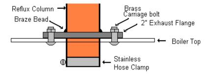
If your boiler doesn't have a removable top then you will not be able to use this method of assembling the column to the boiler.
