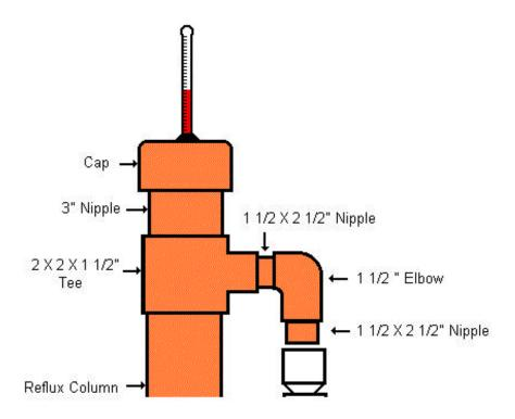
The cap is drilled in the center with a 3/8" hole to fit a rubber grommet and the thermometer stem. Not all stems have the same diameter, so you should make sure the hole fits your thermometer. The cap is <u>not</u> soldered to the column. This is to allow the column and packing to be back flushed and cleaned out by simply taking off the cap and hosing down the column.
