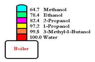
The coolest part of the tower is at the top, and the warmest nearest the heat source at the bottom.
