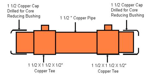
One cap has a 1 1/8" hole drilled in the end, the other cap, a 5/8" hole. The hardest part is to cut the right size holes in the caps so they will fit nicely with the core.
