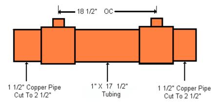
The more important dimension is the overall jacket length. When the core is placed inside the assembly, it should fit snugly at both the top and bottom caps. You can adjust the length of either one of the nipple fittings (before you solder them) to make any fine adjustments.
