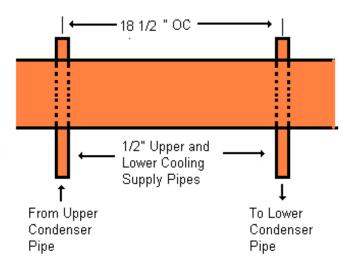
When the holes have been drilled, clean up the top end and solder the Tee fitting, nipple, and the middle section together. Then install the 1 ½" nipples and elbow to the tee connection. Do <u>not</u> solder these yet. They must be left free for final fitting of the condenser assembly.
