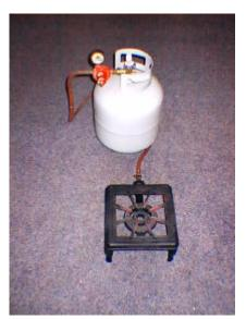
A gas heat source will also react much more quickly to control changes than electric, and is capable of producing far more heat than electrical household circuits can supply.
