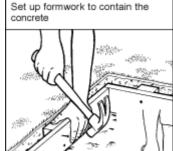
Set up levelled formwork to contain the concrete and check diagonals (1). Then lay thoroughly compacted hardcore and cover with sand.
