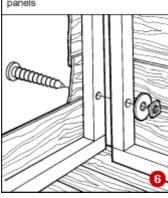
The panels are joined to each other through pre-drilled holes, using screws and washers or nails (6). It is usual to start with a side and back panel, then to add the other side panel, and finish with the door section.
