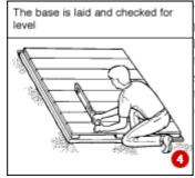
The floor will comprise boards fixed to bearers. It is simply laid in place and will be held there by the weight of the shed. Check with a spirit level that the base is horizontal (4).
