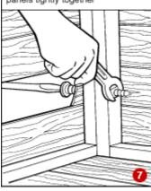
The action of tightening the screws or banging home the nails draws the wall panels together (7). Subsequent panels are secured to each other.
