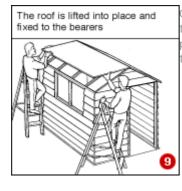
Once the walls are erected, fit the roof (9). The panel or panels are usually fixed to the walls with nails.
