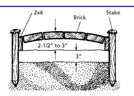
Brick walkway ought to be crowned, as shown in this drawing. Or, the walk should be pitched slightly one way or the other for drainage. The crown or pitch is made with a dragboard; see next page for construction details. Wet the sand to compact it before dragging the board.
