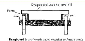
**Dragboard** is two boards nailed together to form a notch for the forms. Curve the board for a crown or pitch with a plane.
