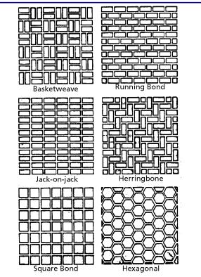
Brick walk patterns are illustrated above. The easiest are jack-on-jack and square bond. The hexagonal design, of course, must be made with hexagonal bricks. Herringbone takes patience. So does the basketweave, as the text details.
