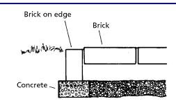
**Brick edging** can be considered standard for brick walkways. The bricks usually are set on a concrete base; the concrete is put in a "trench."
