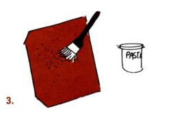
Apply paste generously to the back of the paper, using a good-sized brush.
