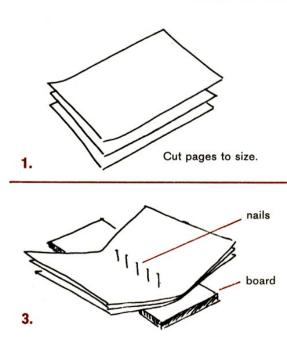
Punch five holes through the fold. The best way to do this is by hammering thin nails through the paper. Use a scrap of wood underneath to protect the top of your work table.
