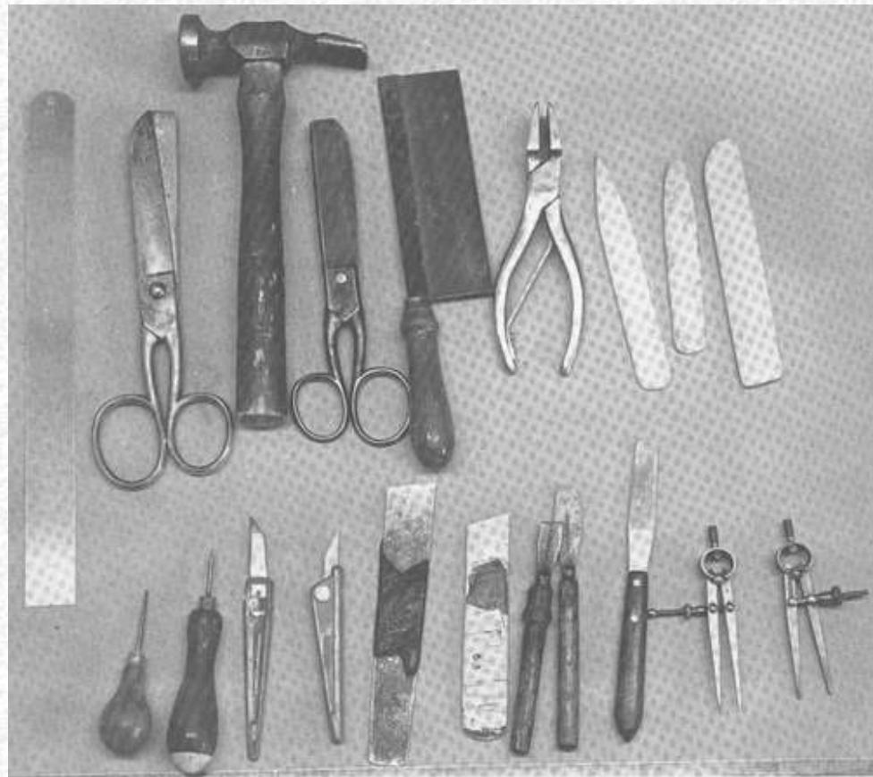
**Figure 2 - Basic took:** top, left to right, metal foot rule, large shears, backing hammer, smaller shears, tenon saw, band nippers, three bone folders; bottom, left to right, two bradawls, two cutting knives, two paring knives, three palette lifting knives, two pairs of dividers.
