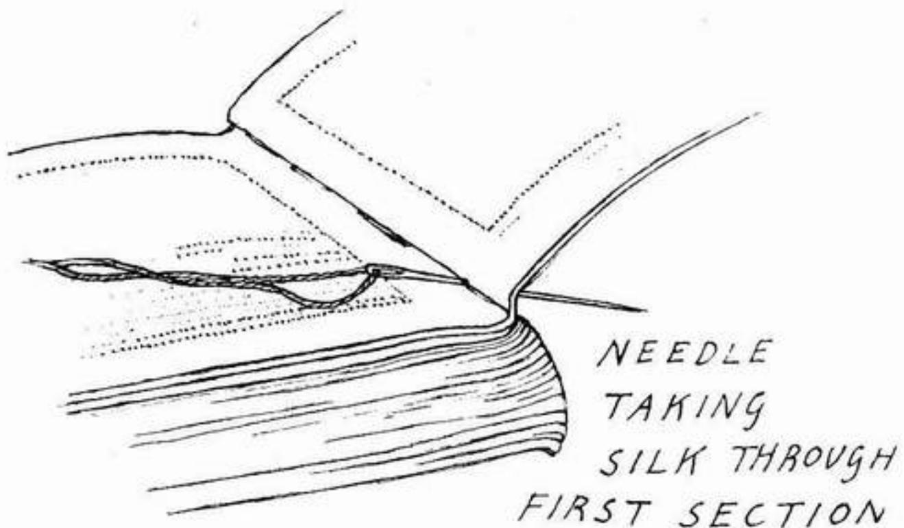
**Figure 28** - *Threading silk for headband*
