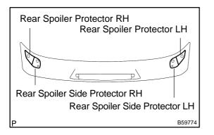
(4) Install 4 new rear spoiler protectors to the rear spoiler as shown in the illustration.
