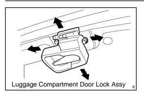
(g) Perform the forward/rearward and right/left adjustments, by loosening the bolts of the luggage compartment door. Torque: 5.5 N-m (56 kgf-cm, 49 in.-lbf)
