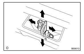
(e) For forward/rearward and right/left adjustments, loosen the bolts.
