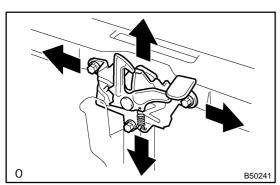
(c) Adjust the lock by loosening the 3 bolts. Torque: 7.0 N-m (82 kgf-cm, 71 in.-lbf)
