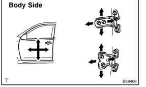
Using SST, adjust the door by loosening the body side hinge bolts.
