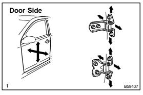
(b) Adjust the door by loosening the door side hinge bolts.
