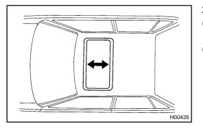
(a) Check the difference in level between the sliding roof weatherstrip and roof panel.
