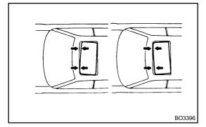
(c) When the front or rear alignment is not correct, remove the drive gear and sliding roof glass, then adjust the drive rail.
