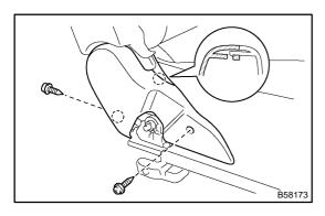
(b) Remove the seat cushion shield inner.
