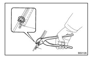
(b) Using hog ring pliers, install the seat cushion cover with new hog rings.
