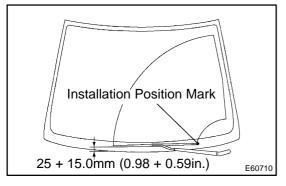
(d) Install the front wiper arm LH with a nut at the position as shown in the illustration.
