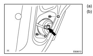
(a) Remove the service hole cover.(b) Remove the 2 nuts and disconnect the connector.
