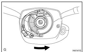
(c) Turn the cable counterclockwise by hand until it becomes harder to turn.
