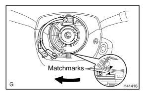
(d) Then rotate the cable clockwise about 2.5 turns to align the marks.
