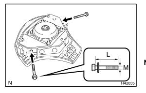
(1) Install the 2 bolts with washers in the 2 bolt holes in the horn button assy.
