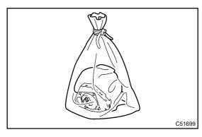
(g) Dispose of the horn button assy (with airbag). **CAUTION:**
