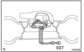
(4) Face the upper surface of the horn button assy upward. Separately tie the left and right sides of the horn button assy to the disc wheel through the hub nut holes. Position the horn button assy connector so that it hangs downward through a hub hole in the disc wheel.
