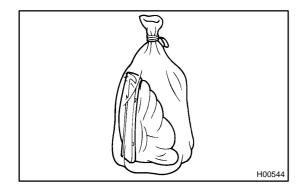
(g) Dispose of the front seat airbag assy.
