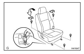
(b) Disconnect the front seat airbag assy connector. **NOTICE:**
