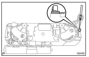
Using a screwdriver, open the claw of the cable clamp and (b) disconnect the defroster damper control cable.
