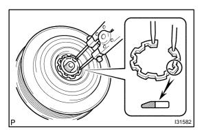
(d) Using a snap ring expander, install the magnet clutch rotor and a new snap ring with the chamfered side facing up.
