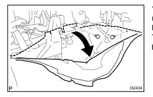
REMOVE AIR DUCT REAR NO.4 (W/ COLD AREA) 12.
