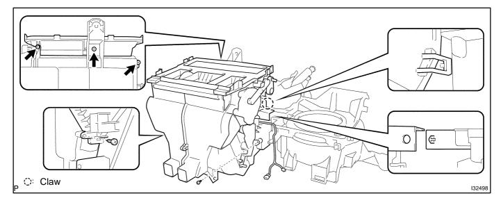
(c) Install the heater case with the claw and 2 screws.
