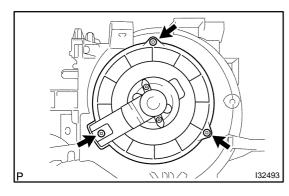
26. REMOVE BLOWER W/FAN MOTOR SUB-ASSY
