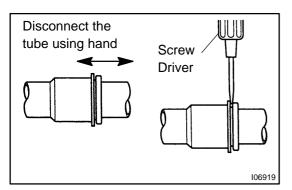
(e) Disconnect the cooler refrigerant suction hose No. 1. **NOTICE:**
