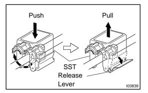
(b) Push down SST and release the clamp lock. **NOTICE:**
