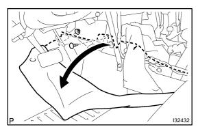
8. REMOVE INSTRUMENT PANEL BRACE SUB-ASSY NO.1
