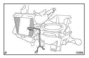
(d) Remove the cooler thermistor No. 1 from the cooler evaporator sub–assy No. 1.
