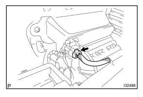
(d) Disconnect the connector from the cooler thermistor No. 1.
