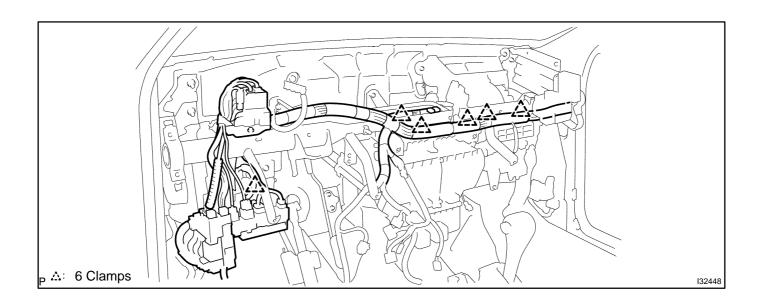
(c) Remove the 6 bolts and instrument panel reinforcement.
