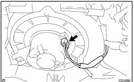
(b) Disconnect the connector from the blower w/ fan motor sub-assy.
