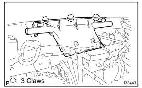
15. REMOVE DEFROSTER NOZZLE ASSY(a) Release the 3 fitting claws, remove the defroster nozzle
