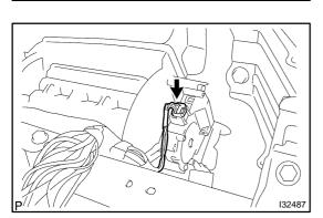
(c) Connect the connector to the damper servo sub-assy.
