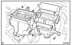
(e) Remove the 4 nuts, bolt and air conditioner unit assy.
