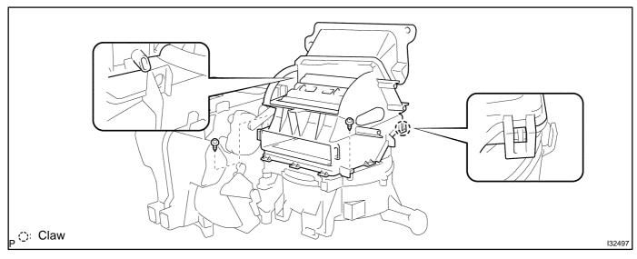
(c) Release the fitting claw, remove the 5 screws and heater case.
