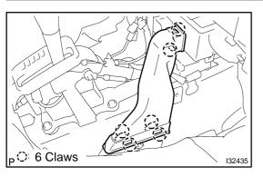
(b) Release the 6 fitting claws, remove the air duct rear No.4.
