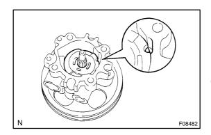
(c) Align the dent of the vane pump side plate front with that of the vane pump housing front, and install the vane pump side plate front.
