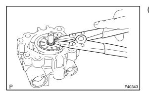
(d) Using a snap ring expander, install a new snap ring to the w/ pulley shaft sub–assy.
