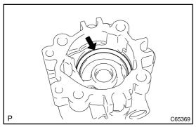
(c) Remove the O-ring from the pump housing front.
