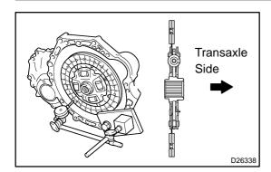
(c) Using a dial indicator, check the clutch disc assy runout.
