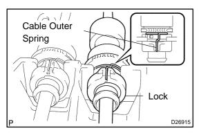
(e) Connect the shift cable to the retainer of shift lever assy, turn the lock.
