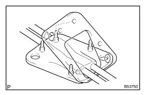
(i) Remove the retainer from the grommet.
