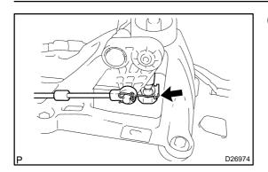
(f) Separate the end of the shift cable from the shift lever assy.
