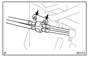
(c) Remove the 2 nuts and clamp.
