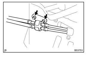
(c) Remove the 2 nuts and clamp.
