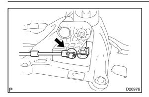
(f) Separate the end of the select cable from the shift lever assy.
