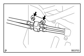
(g) Install the clamp with the 2 nuts.
