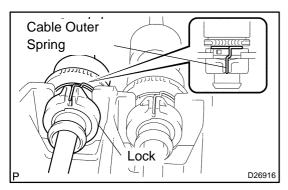
(e) Connect the select cable to the retainer of shift lever assy, turn the lock.
