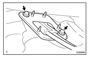
(c) Install the control cable assy with the 2 bolts.
