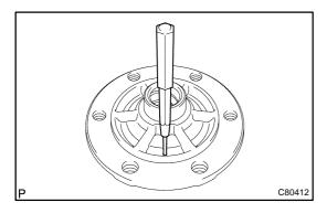
(b) Using a pin punch (φ 3 mm) and a hammer, remove the front differential pinion shaft straight pin from the front differential case.
