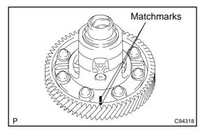
(c) Align the both matchmarks, quickly install the 8 bolts with the front differential ring gear to the front differential case.
