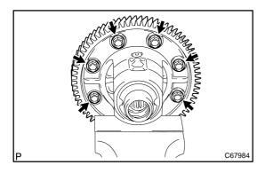
(b) Remove the 8 bolts. Using a hammer, remove the front differential ring gear.
