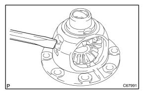
(b) Using a chisel and a hammer, stake the front case hole.
