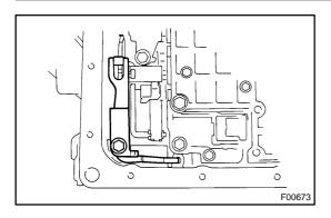
(b) Remove the bolt and manual detent spring.
