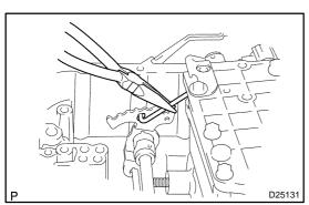
(d) While disconnecting the manual valve connecting rod from the manual valve lever, remove the valve body with the manual valve together.
