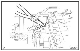
(e) While connecting the manual valve connecting rod to the manual valve lever, install the valve body with the manual valve together.
