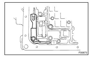
(g) Install the manual detent spring and bolt.
