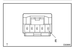
(b) Using an ohmmeter, measure the resistance at terminal E (1) and body ground.
