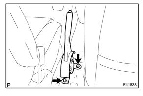
(c) Install the parking brake lever with the 2 bolts.
