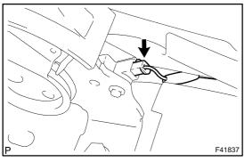
(d) Connect the parking brake switch connector to the parking brake switch.
