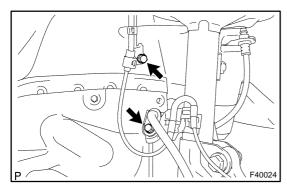
(c) Remove the 2 clamp bolts holding the sensor harness from the body and shock absorber.
