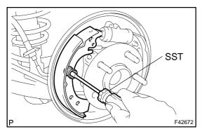
(b) Using SST, install the front brake shoe, pin, shoe hold-down spring and cup.
