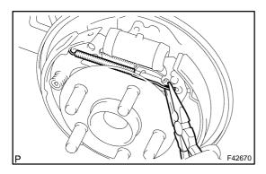
(b) Using a needle–nose pliers, install the upper side tension spring.
