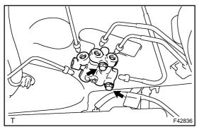
(b) Remove the 2 bolts and proportioning valve assy from the body.
