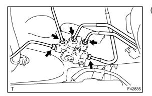
(b) Using SST, connect the 5 brake tubes to the proportioning valve assy.
