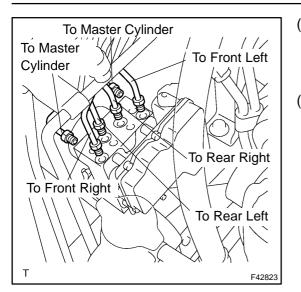
(b) Using SST, connect the 6 brake tubes to the correct position of brake actuator, as shown in the illustration.
