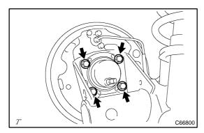
15. INSTALL REAR AXLE HUB & BEARING ASSY LH
