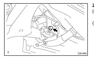
21. FULLY TIGHTEN REAR AXLE BEAM ASSY(a) Fully tighten the bolt.
