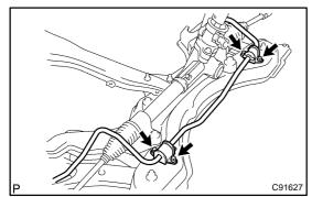
(b) Install the stabilizer bar front and 4 bolts to the front suspension crossmember sub-assy.
