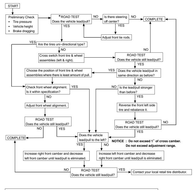
Select a flat road where the vehicle can be driven in a straight line for 100 meters at a constant speed of 35mph. Please confirm safety and set the steering wheel to its straight position. Drive the vehicle in a straight line for 100 meters at a constant speed of 35 mph without holding the steering wheel.
