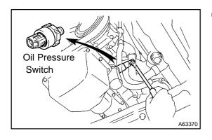
(b) Using a 24 mm deep socket wrench, remove the oil pressure switch.
