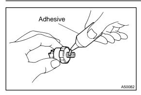
(f) Apply adhesive to 2 or 3 threads of the oil pressure switch. **Adhesive:**
