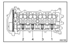
(g) Loosen the bearing cap bolts on camshaft in the order as shown in the illustration in several passes, then remove the bearing caps.
