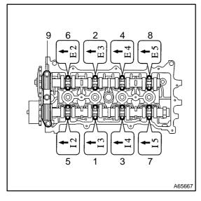
(c) Examine the front marks and numbers, then tighten the bolts in the order shown in the illustration.
