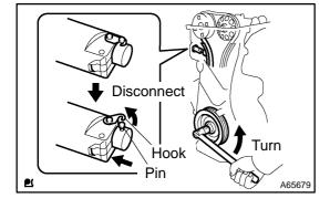
(c) Turn the crankshaft counterclockwise, then disconnect the plunger knock pin from the hook.
