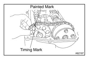
(o) Put the camshaft No. 2 on the cylinder head with the painted mark of the chain aligned with the timing mark on the camshaft timing gear.
