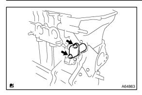
(c) Remove the 2 nuts and chain tensioner.
