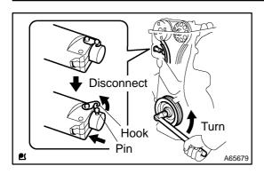
(4) Turn the crankshaft counterclockwise, then disconnect the plunger knock pin from the hook.
