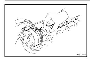
(h) Remove the camshaft while holding the chain.
