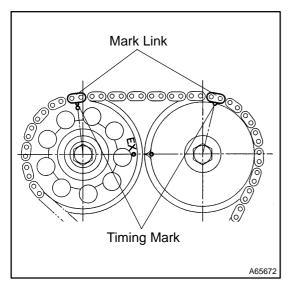
(d) Install the chain on the camshaft timing gears with the yellow color mark links aligned with the timing marks on the camshaft timing gears.
