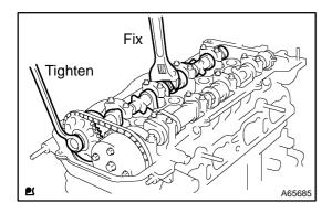
(r) Fix the camshaft with a spanner and so on, then tighten the camshaft timing gear set bolt.
