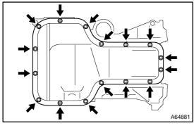
(c) Install the oil pan with the 14 bolts and 2 nuts.
