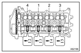
(n) Examine the front marks and numbers, then tighten the bolts in the order shown in the illustration.
