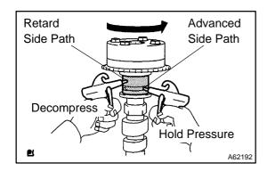
(e) Confirm if the camshaft timing gear assembly revolves to the timing advance direction when weakening the air pressure of the timing retard path.
