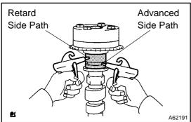
(d) Put air pressure into two broken paths (the advance side path and retard side path) with about 150 kPa {1.5 kgf/ cm²}.
