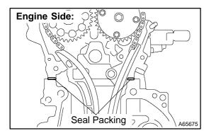
(c) Apply a continuous bead (3.5 to 4.5 mm (0.138 to 0.177 in.) diameter) of seal packing as shown in the illustration.Seal packing:
