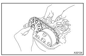
(f) Remove the camshaft timing gear as shown in the illustration.
