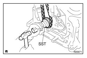
(c) Using SST, install the crankshaft timing gear. SST 09223–22010
