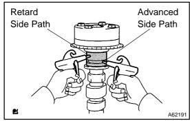
(3) Put air pressure into two broken paths (the advance side path and retard side path) with about 150 kPa {1.5 kgf·cm²}.
