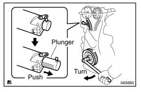
(d) Turn the crankshaft clockwise, then check that the slipper is pushed by the plunger.
