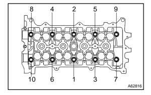
(c) Using a bi–hexagon wrench 10, install and uniformly tighten the 10 cylinder head bolts with the plate washers, in several passes, in the sequence shown.
