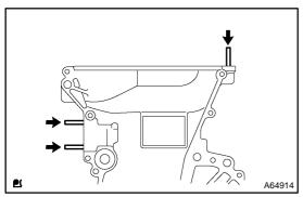
(c) Using a torx socket wrench E5, remove the 3 stud bolts.
