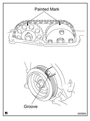
(s) Check the painted marks on the chain and camshaft timing gears. Then, check that the crankshaft pulley groove and the timing mark of the timing chain cover are aligned as shown in the illustration.
