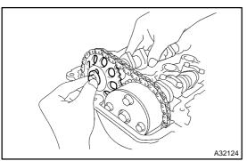
(p) Raise the camshaft, then tighten the set bolt temporarily.
