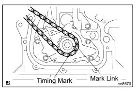
(b) Install the chain on the crankshaft timing gear with the yellow color mark link aligned with the timing mark on the crankshaft timing gear.
