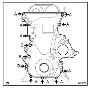
(d) Install the timing chain cover with the 12 bolts and nut. **Torque:**
