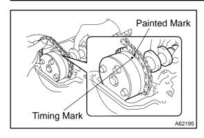
(m) As shown in the illustration, install the chain on the camshaft timing gear with the painted mark aligned with the timing mark on the camshaft timing gear.
