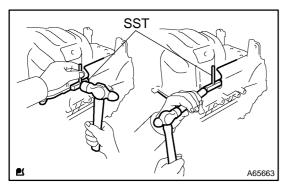
(b) Insert the blade of SST between the bearing cap and oil pan, then cut off the applied sealer and remove the oil pan.
