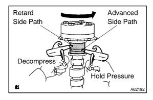
(4) Confirm if the camshaft timing gear assembly revolves to the timing advance direction when weakening the air pressure of the timing retard path.
