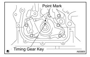
(2) Using a crankshaft pulley bolt, turn the crankshaft to align the timing gear key with the point mark located on the oil pump.
