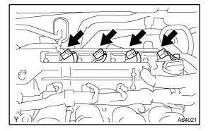
(c) Remove the bolt and nut installing the engine wire.
