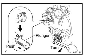
(d) Turn the crankshaft clockwise, and check that the slipper is pushed by the plunger.
