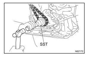
(c) Using SST, install the crankshaft timing sprocket. SST 09223–22010
