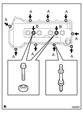
(c) Install the cylinder head cover and 3 cable brackets with the 9 bolts, 2 seal washers and 2 nuts. Uniformly tighten the bolts and nuts, in the several passes.
