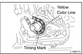
(b) Install the timing chain on the crankshaft timing sprocket with the yellow color link aligned with the timing mark on the crankshaft timing sprocket.
