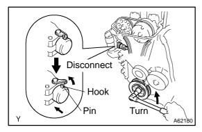
(c) Turn the crankshaft counter clockwise, and disconnect the plunger knock pin form the hook.
