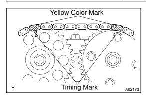
(d) Install the timing chain on the camshaft timing sprockets with the yellow color links aligned with the timing marks on the camshaft timing sprockets.
