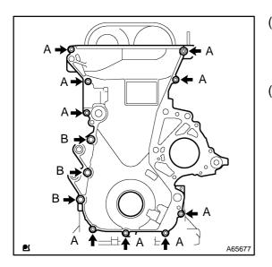
(c) Install the timing chain cover with the 11 bolts and nut. **Torque:**
