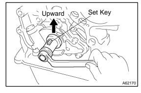
(2) Using a crankshaft pulley bolt, turn the crankshaft and set the set key on the crankshaft upward.
