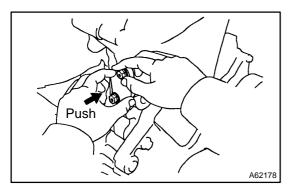
(b) Apply engine oil to the chain tensioner and install it withe 2 nuts.
