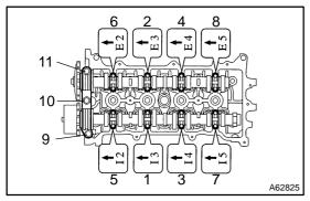
(c) Examine the front marks and numbers and tighten the bolts in the order shown in the illustration.
