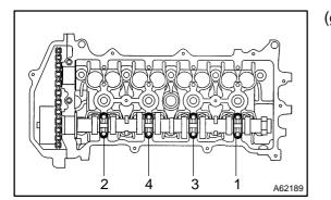
(g) Loosen the camshaft bearing cap bolts on camshaft in the order as shown in the illustration in several passes, and remove the caps.
