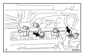
19. INSTALL CYLINDER HEAD COVER SUB-ASSY
