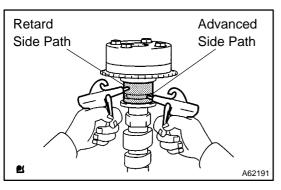
(i) Tie the timing chain with a string as shown in the illustration.
