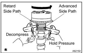
(4) Confirm if the camshaft timing gear assembly revolves in the timing advance direction when weakening the air pressure of the timing retard path.
