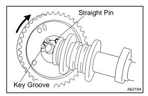
(d) Put air pressure into two broken paths (the advance side path and the retard side path) with about 150 kPa {1.5 kgf·cm}.
