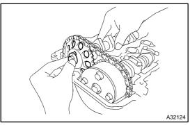
Put the camshaft No.2 on the cylinder head with the (c) painted links of the chain aligned with the timing mark on the camshaft timing gear.
