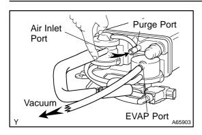
(5) While holding the air inlet port closed, apply vacuum (3.43 kPa, 25.7 mmHg, 1.01 in.Hg) to the EVAP port and check that air flows into the purge port.
