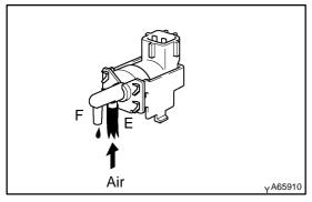
(3) Check that air does not flow from ports E to F.
