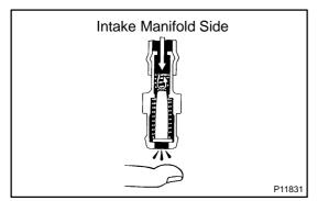
(2) Blow air into the intake manifold side, and check that air passes through with difficulty.
