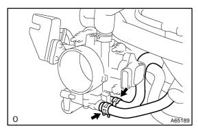
(e) Connect 2 water by-pass hoses to the throttle body.
