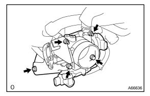
(d) Install the throttle body with 3 bolts and 2 nuts.(Transaxle A/T)
