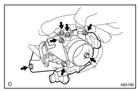
(e) Remove 5 bolts, 2 nuts, throttle body bracket and throttle body. (Transaxle M/T)
