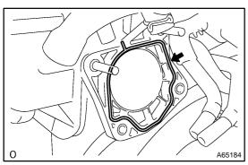
(b) Install a new gasket on the intake manifold, as shown in the illustration.
