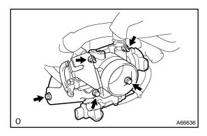
(f) Remove 3bolts, 2nuts and throttle body. (Transaxle A/T)
