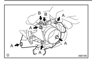
(c) Install the throttle body with 5 bolts and 2 nuts.(Transaxle M/T)
