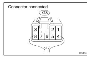
(a) Check the continuity and voltage of the glass breakage sensor ECU, as shown in the illustration and table.
