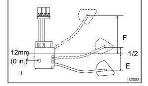
(a) Disconnect the connector fuel sender gauge.
