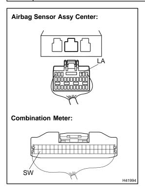
(a) For the connector (on the airbag sensor assy center side) between the combination meter and the airbag sensor assy center, measure the resistance between SW and LA.
